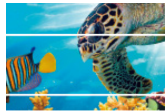
Gap/White streaks (Excessive feeding amount)
