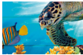
Overlap/Black streaks (Insufficient feeding amount)
